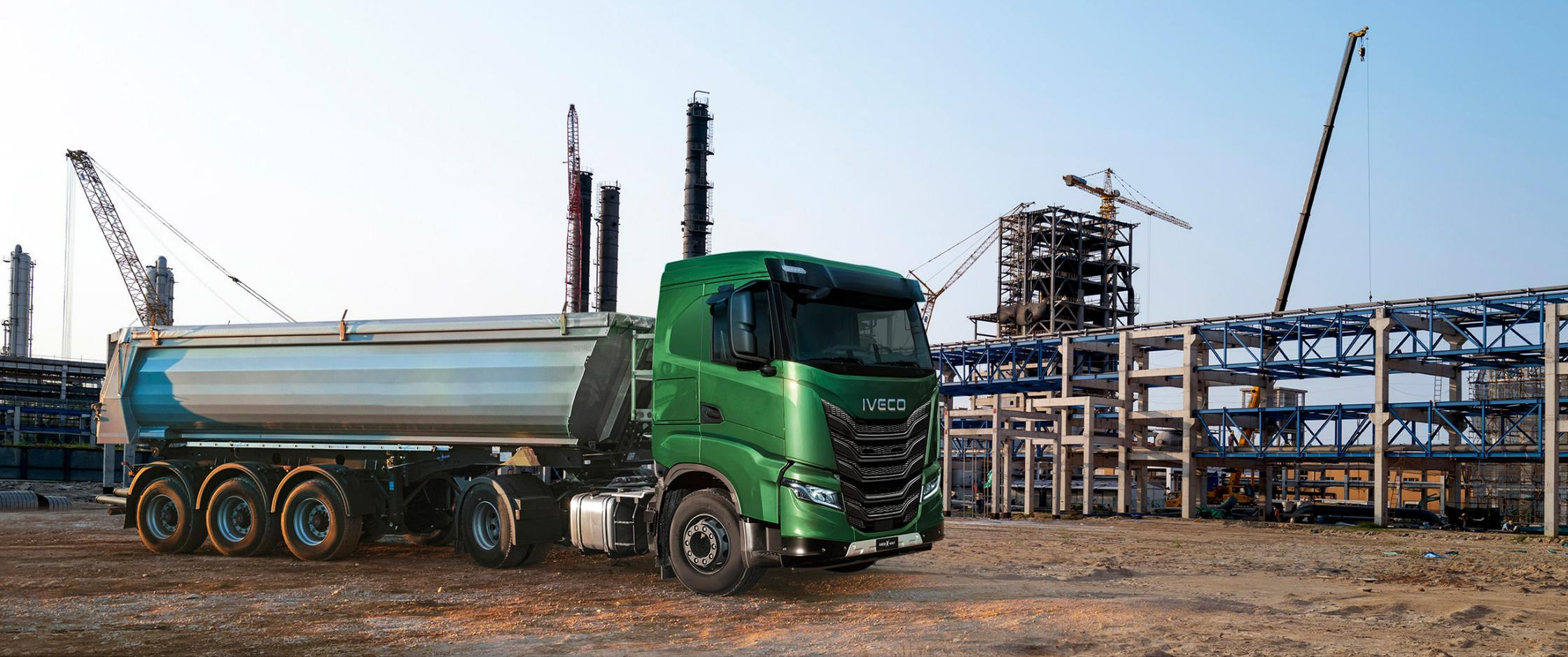
XCursor 13 Natural Gas version produces 500 hp and 2.200 Nm of torque while achieving up to 10% in fuel consumption reduction. This powerful performance comes with the environmental advantages of Natural Gas, which can help to significantly reduce vehicle emissions, with up to 90% reduction in CO<sub>2</sub> when run on biomethane.
